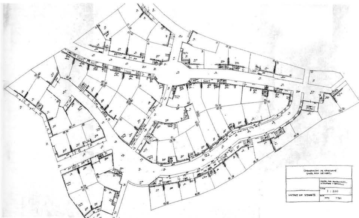
FIG. 5A AND 5B Stakes for house lots, streets, and building masses in a neighborhood in Santa Rosa de Cabal, Columbia, and the site plan arising from this process. All these stakes were placed by family members themselves with help and guidance from Center for Environmental Structure staff.
